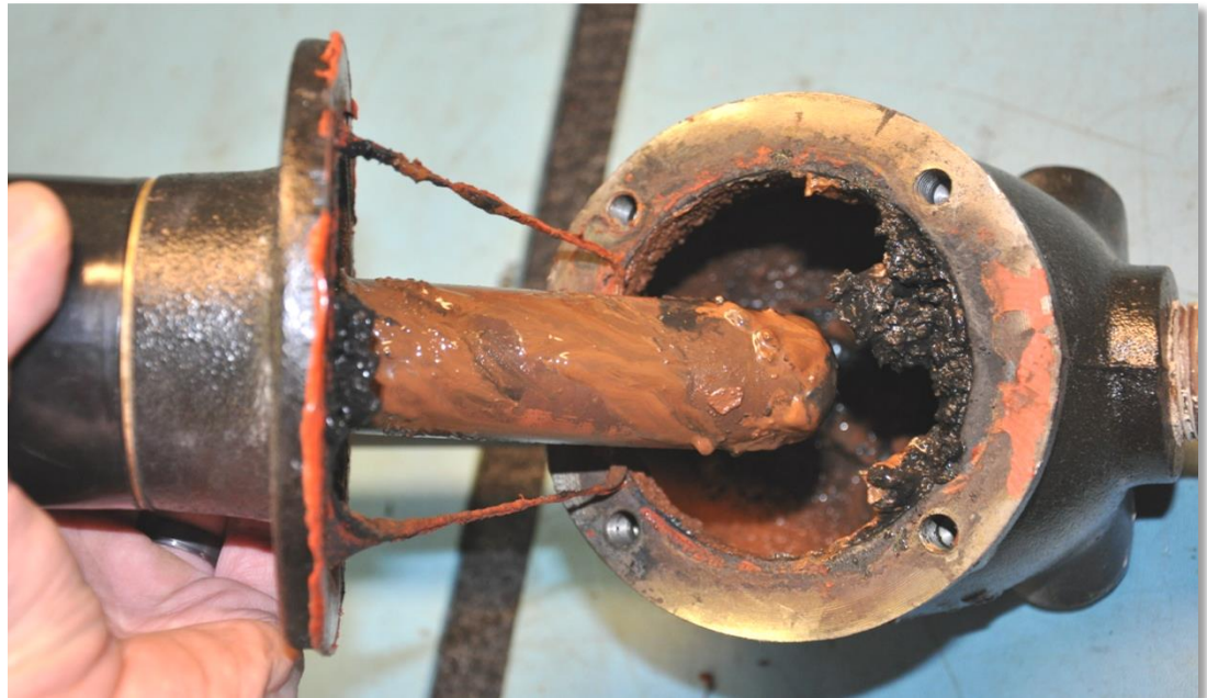
Figure 2: Float style low water cutoff switch that failed due to excessive build-up of sludge
